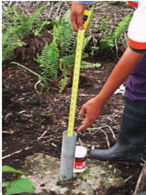
Figure 7-6: Example of piezometer for measuring groundwater levels.
