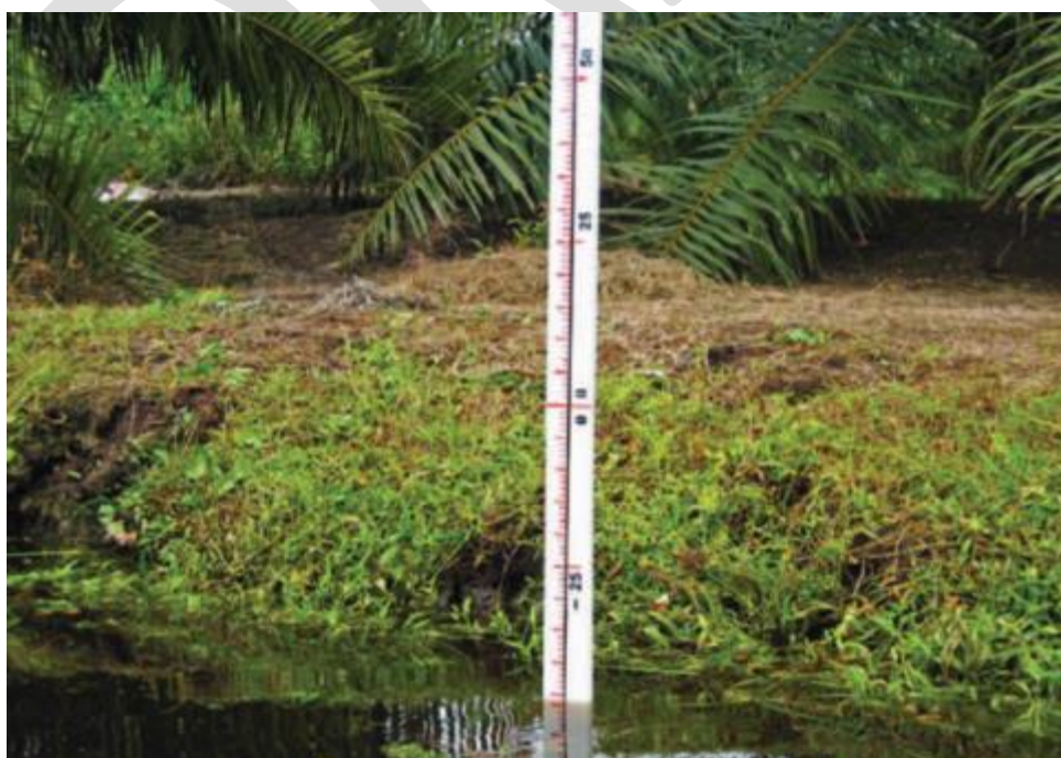
Figure 7-5: Water level gauge for water level monitoring in collection drain.
