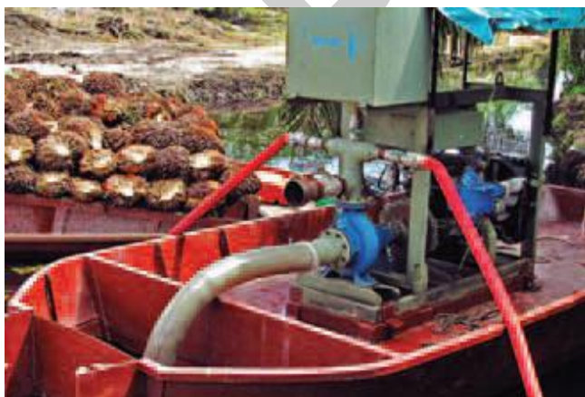
Figure A5-1: Close up example of fire boat used for fire suppression activities in oil palm plantations on peatland.
