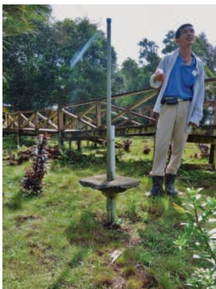
Figure 7-1: Example of subsidence pole installed together with a piezometer. Peat subsidence over time in this site is clearly visible.
