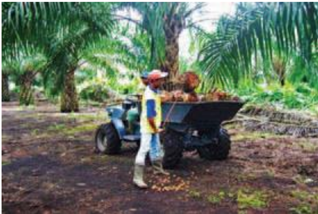
Figure 5-8: Low ground pressure (LGP) tyres on compacted path.
