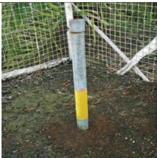
Figure 7-2: Photo in 2010 of a subsidence pole installed in late 2007, 10 years after initial drainage.
