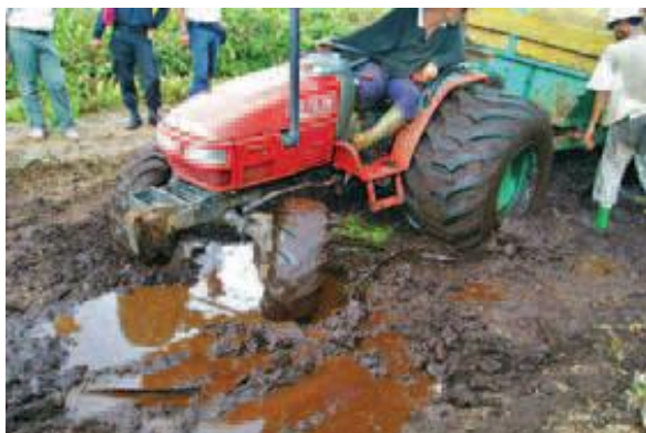
Figure 5-5: Operational problems encountered when ground bearing capacities of deep peat are exceeded.
